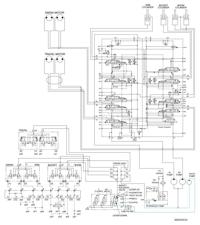
When the knob of the safety solenoid valve is moved downward, oil flows into the remote control valve through line filter, safety solenoid valve and corss assy.
