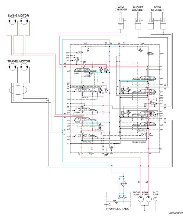
When the swing and arm functions are operated, simultaneously the swing spool and arm spools in the main control valve are moved to the functional position by the pilot oil pressure (pa2, pb2, pa5, pa9, pb5, pb9) from the remote control valve.
