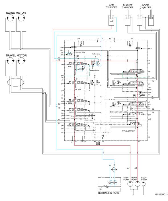
When the LH control lever is pulled back, the arm spools in the main control valve are moved the to roll in position by the pilot oil pressure (pa5, pa9) from the remote control valve.
