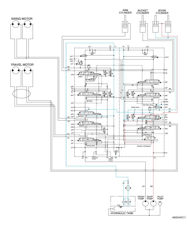
When the RH control lever is pushed forward, the boom spools in the main control valve are moved to the down position by the pilot oil pressure (pb3, pb7) from the remote control valve.
