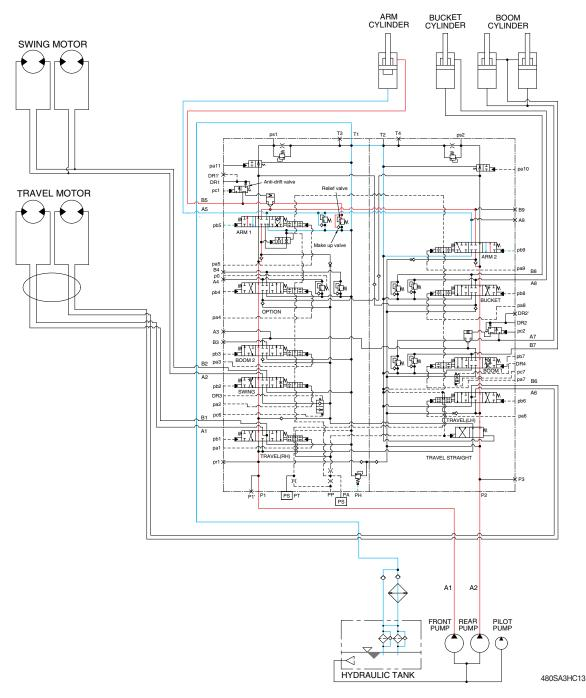
When the LH control lever is pushed forward, the arm spools in the main control valve are moved to the roll out position by the pilot oil pressure (pb5, pb9) from the remote control valve.
