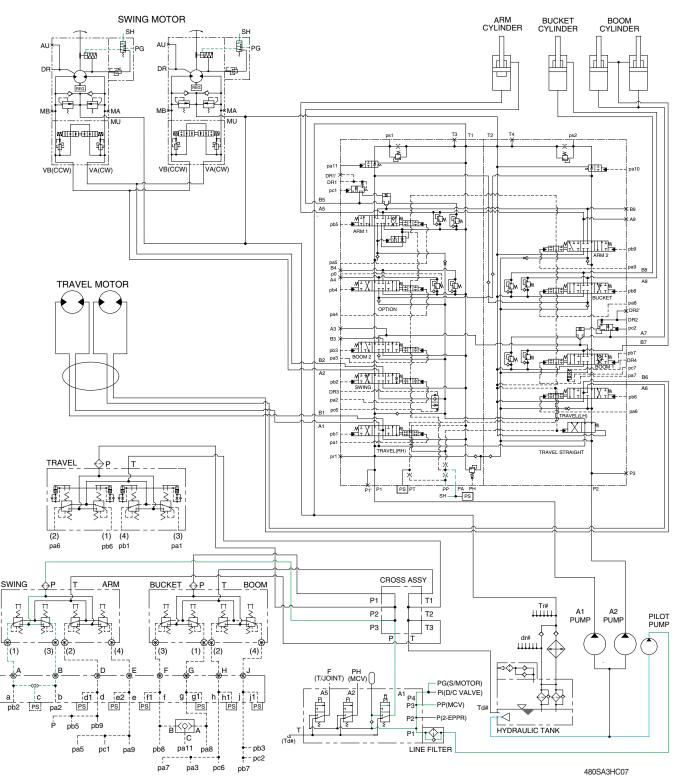
When one of the RCV lever (except travel lever) is tilted, the pilot oil flows into SH port through main control valve.
