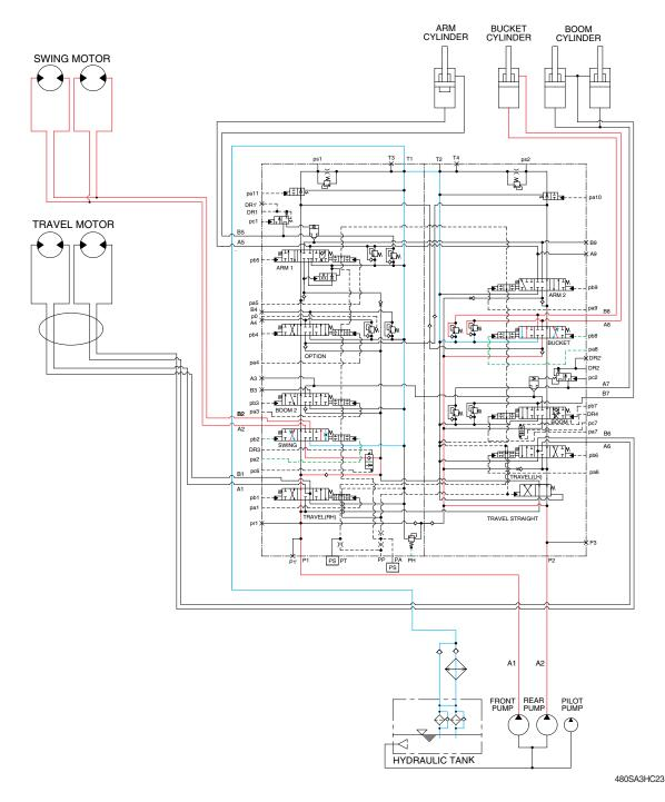
When the swing and bucket functions are operated, simultaneously the swing spool and bucket spool in the main control valve are moved to the functional position by the pilot oil pressure (pa2, pb2, pa8, pb8) from the remote control valve.
