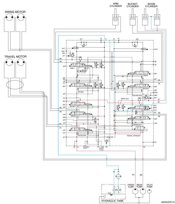
When the RH control lever is pulled back, the boom spools in the main control valve are moved to the up position by the pilot oil pressure (pa3, pa7) from the remote control valve.
