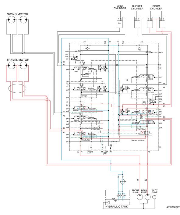
When the boom and travel functions are operated, simultaneously the boom spools and travel spools in the main control valve are moved to the functional position by the pilot oil pressure (Pa3, pa7, pb3, pb7, pa1, pb1, pa6, pb6) from the remote control valve and the straight travel spool is pushed to the right by the oil pressure from pilot pump.
