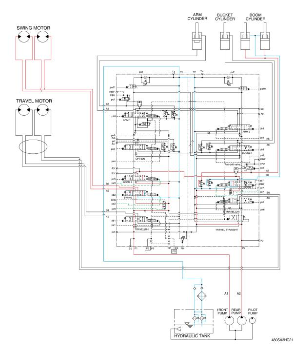
When the swing and boom up functions are operated, simultaneously the swing spool and boom spools in the main control valve are moved to the functional position by the pilot oil pressure (pa2, pb2, pa3, pa7) from the remote control valve.
